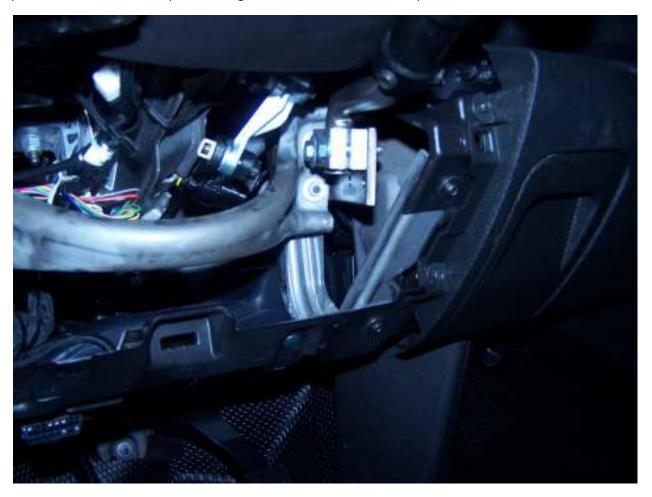
Notice how the support rod needs to be bent in order to exit the dash properly.
