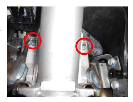
Slide the holes on the arms of the bracket over the studs. When the bracket is in place, reattach the two nuts and tighten them down to OEM standards. Once the bracket is in place you can move on to mounting the support rod.
