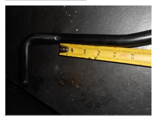
Install the brake rod, brake tube assembly and gas rod with supplied 7010-17 gas block to gas pedal rod, bend gas tube to desired shape and finalize installation!
